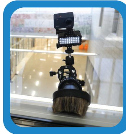
All pieces will screw or thread together. Be sure to tighten each section sufficiently so that it doesn't move while you're working. If you need to change the angle of the camera or light, simply loosen the screw(s) to adjust the angle and retighten. The camera threads onto the top piece but may be facing the wrong direction. Loosen the camera to face the direction you desire and then turn the dial on the connector piece to tighten.
