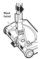
The swivel, located on the POWERHEAD allows you to turn the handle to the left side to reach farther under low furniture.
